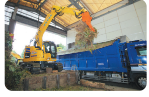
PC138USE 有線式電動仕様 Wired electric hydraulic excavator
