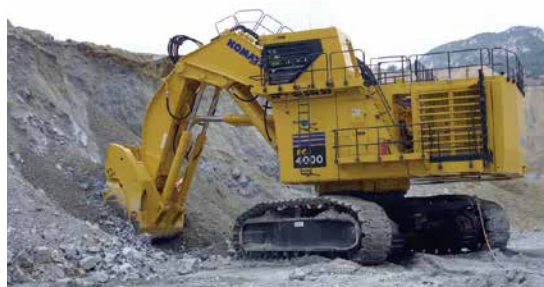
PC4000 mining shovel (bucket capacity: 22 cu. meters or 29 cu. yards)
