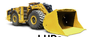
LHDs (load, haul, dump machines)
