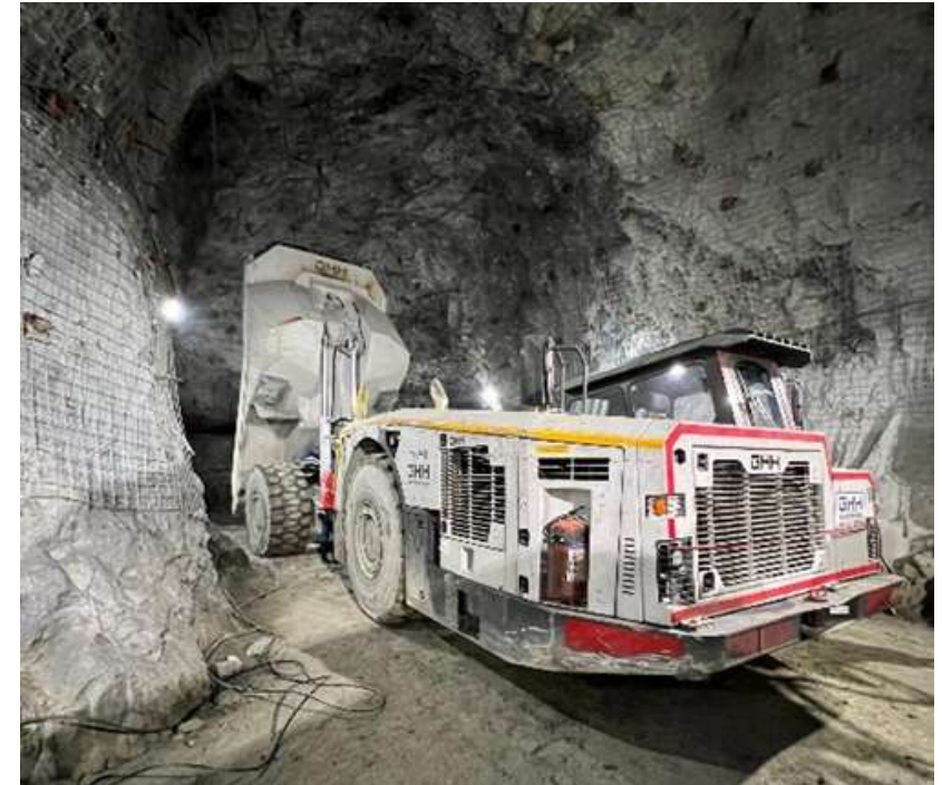
GHH-made MK-42 underground dump truck
