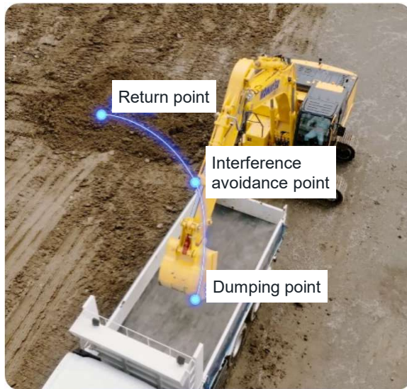
Auto swing function in loading work achieves easy work for lower skill operators.
