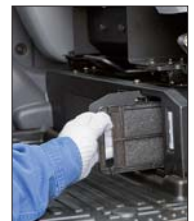
Internal air conditioner filter
