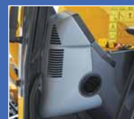
Defroster (Conform to the ISO 10263-5 standard)
