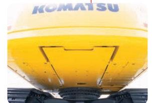
Strengthened revolving frame undercover
