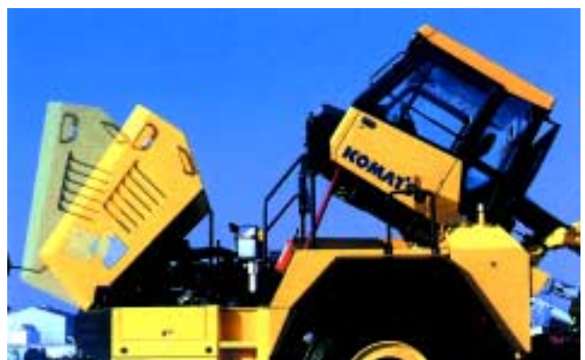
Fig. 12 Fully opening hood and tiltable cab
