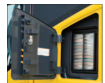
External air conditioner filter
