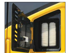
External air conditioner filter
