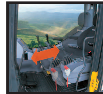
Seat Sliding Amount: 340 mm 13.4", increased 120 mm 4.7"
